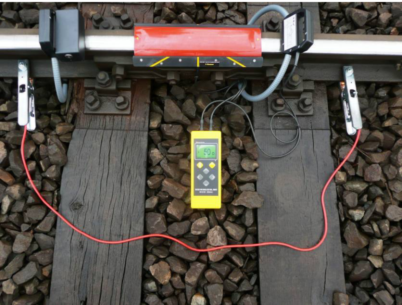
Fig. 3.2 SICO 2046 with parallel short circuit
