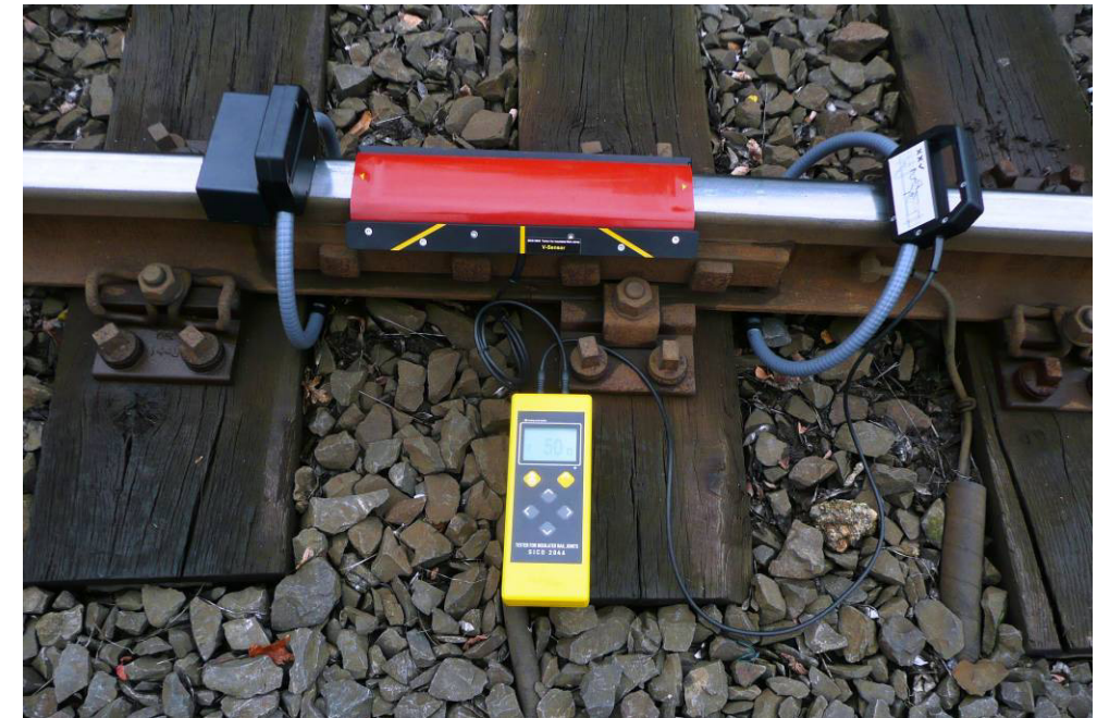
Fig. 3.4 C-sensor located before the next conductor branching off
