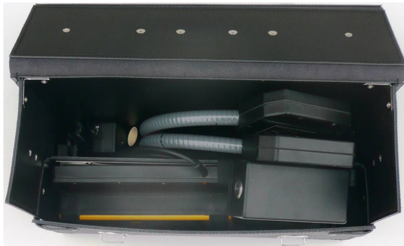
Fig. 2.2 Transport case with insulated rail joint tester
