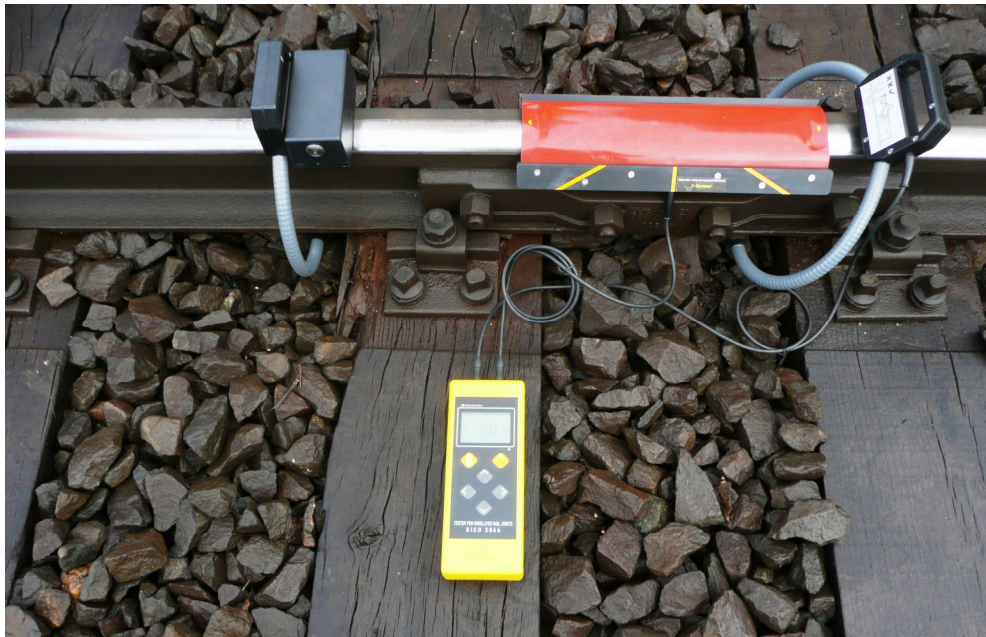
Fig. 3.8 C-sensor looped around rail and joint
