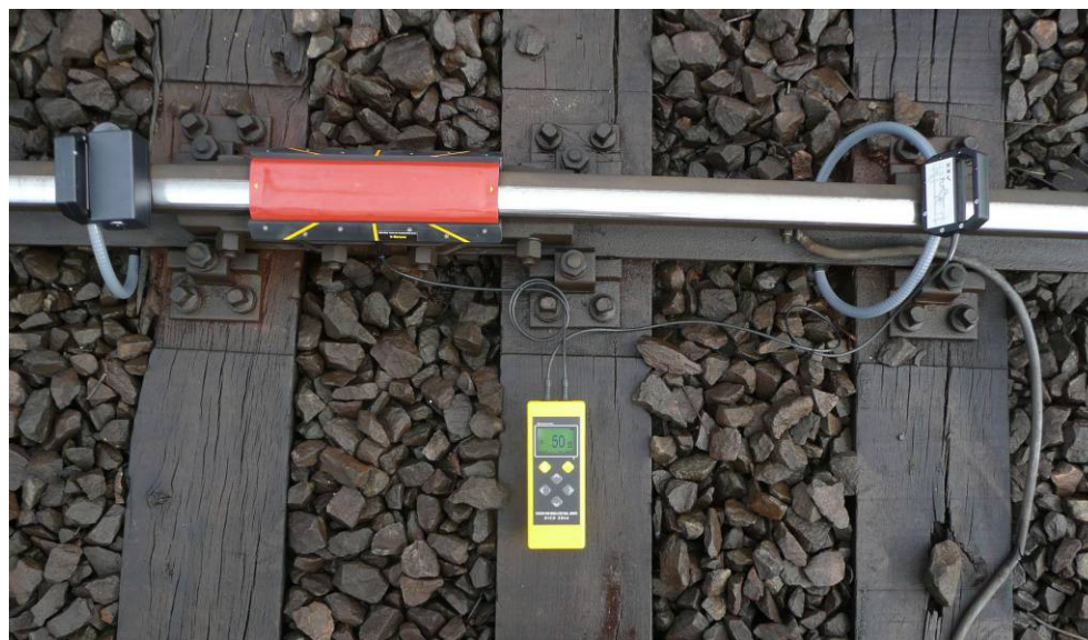
Fig. 3.7 C-sensor looped around rail and a conductor
