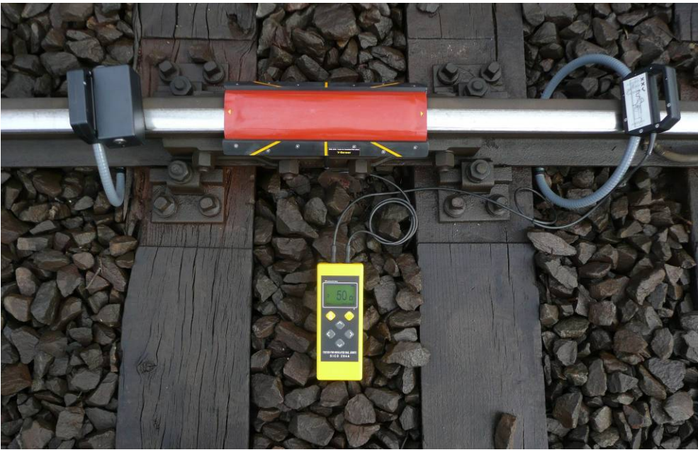
Fig. 3.9 C-sensor located next to the sleeper
