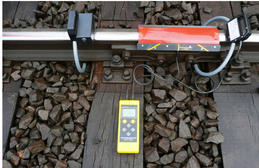
Fig. 3.6 C-sensor looped around rail and joint
