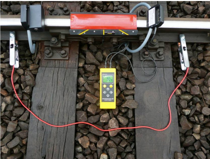
Fig. 3.2 SICO 2046 with parallel short circuit
