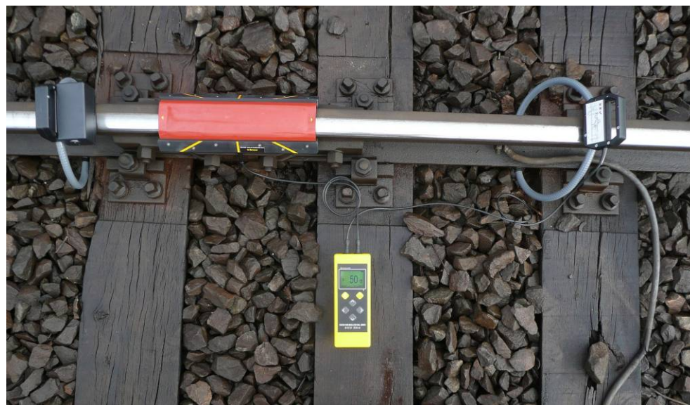
Fig. 3.7 C-sensor looped around rail and a conductor
