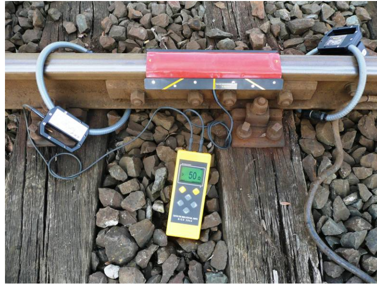
Fig. 3.1 Assembly SICO 2046 on rail
