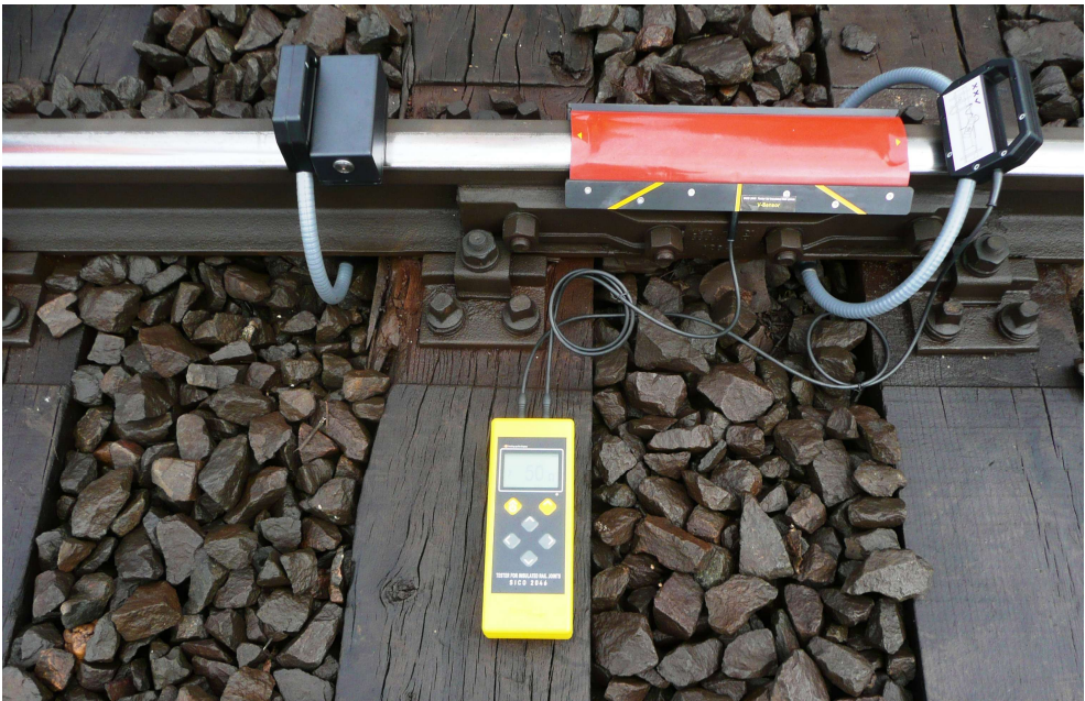
Fig. 3.8 C-sensor looped around rail and joint
